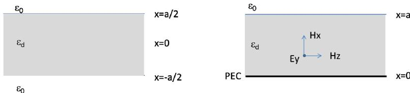
8. Rectangular Waveguide TE<sub>10</sub> mode (20 points)
